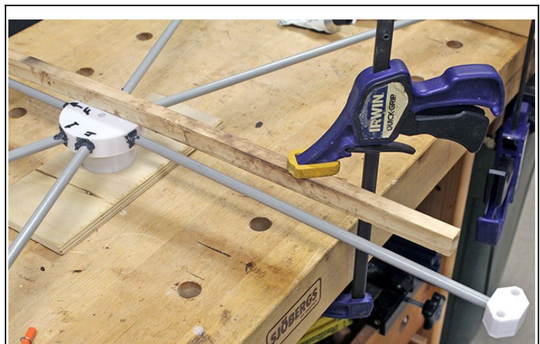
Figure 9: Clamping the hub to the workbench
